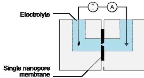
**Figure 1.** Schematic of cell for measurement of nanopore current–voltage characteristics.
