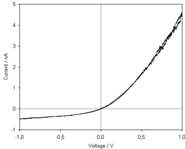
**Figure 2.** Rectification of current through a nanopore. Current is the average of five voltage scans over  $\pm 1$  V.
